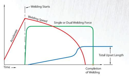
The welding energy is infinite coming from a Direct Drive motor. Parameters (variables) are: RPM, Friction and Forge Force, Time and Distance, and Breaking Time. This weld process is best applied for solid diameter bars up to 250 mm. To improve weld quality, the spindle can turn during the forge phase. Flash turning is easier than on an Inertia welder.
