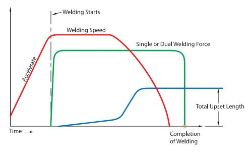
This variation combines the infinite weld energy source of Direct Drive with the flywheel effect of Inertia. It is best applied for pre-heat on materials which need slower post-weld, cooling rates or materials which are brittle at ambient temperatures. The Hybrid process is also used for various super-alloy combinations such as large ship diesel valves or turbochargers.
