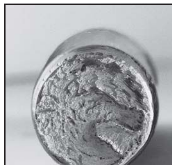
Induced failure showing typical classic Direct Drive Friction Weld flow pattern.
