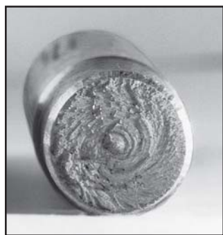
Induced failure showing helical flow on an Inertia Friction Weld.
