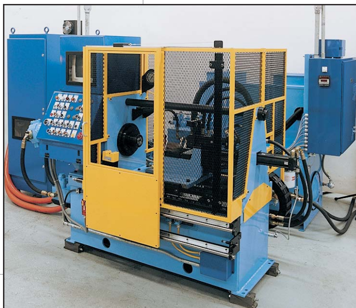
Below: Model 120B Inertia Friction Welder with safety guarding installed.
