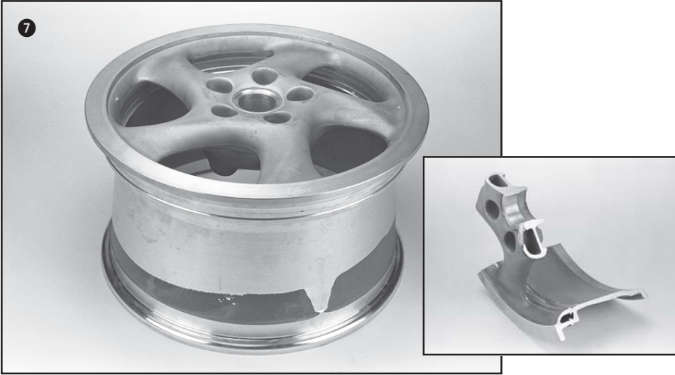
7 Aluminum wheel rim and cross-section.
