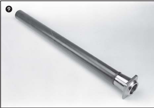
9 Rear axle housing tube. Forged tube end welded to tube stock.
