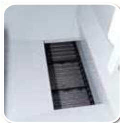
Drainage outlet & Chip conveyor
