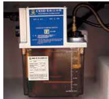
The automatic lubrication pump is installed at low level for easy monitoring.
